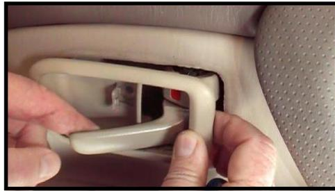
8. Remove electrical window control panel using flat screw driver and a plastic ruler or Interior trim tool.
