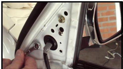
15. Do not touch the screw in the centre. This screw helps support the mirror whilst you are removing bolts. Once the bolts have been removed lift the mirror and carefully remove and feed electrical cable through the door frame.
