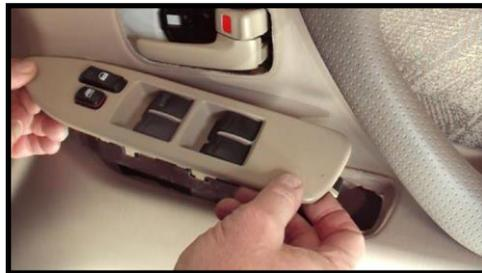
9. Remove the wire plug behind the electrical window control panel by pressing down on the small tag.
