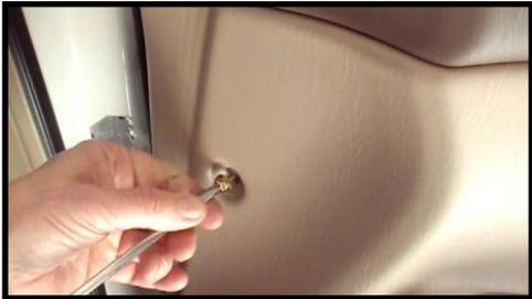
5. Remove triangular plastic cover at the "hinge end" covering the mirror bolts. It will detach with some firm manual pressure.
