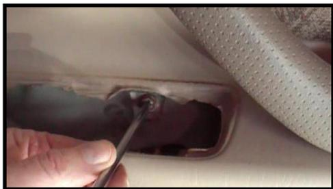
11. Remove 2 plastic pins at “latch end” and 1 at the “hinge end”. Use Phillips screw driver to pop inside button then remove using your fingernails to lift them out.
