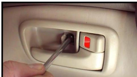
7. Remove door latch outer cover with flat screw driver. Loosen top first, then the bottom.
