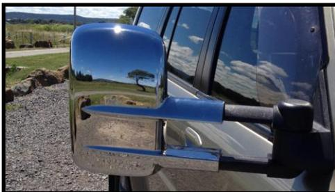
The Mirrors are designed to offer the best for viewing from the driver's position. However they will fold in if you accidentally strike an object or need greater clearance.
