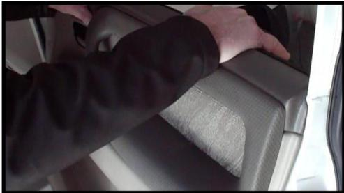
20. Replace the 2 plastic pins at the "latch end" then the single pin at the "hinge end". Hint: prepare the pin by pushing the shaft through past the head. Then press it back into the hole, and press the centre pin until flush.
