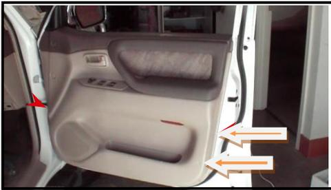
12. All the screws and pins connecting the door cover should now be removed. Tap underneath the door cover with the palm of your hand until the top separates from the window cavity. Then remove the door panel.
