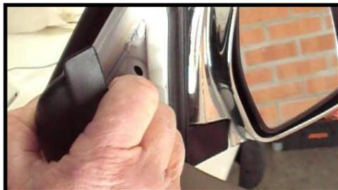
6. Door handle: Pop out the screw cover by wedging in a flat screw driver. Remove screw behind the cover.
