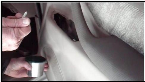
21. Replace the two screws and plastic caps at the "hinge end" on the door.
