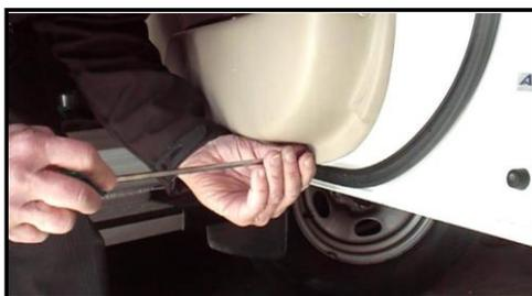
3. Remove 2 plastic caps at "hinge end". They will pop out easily with a flat screw driver or interior trim tool.
