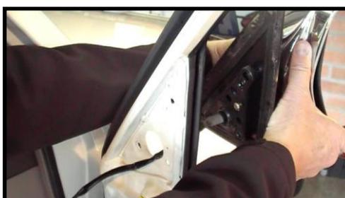
16. Seat the Towing Mirror in place, ensuring that the rubber seal is flush and in position.
