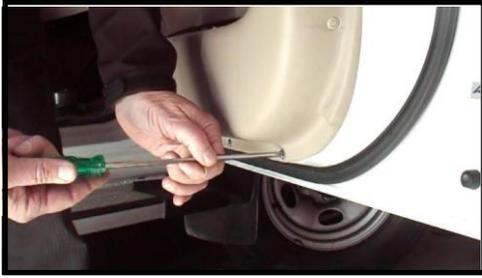
23. Replace the door handle cover. Then replace the screw behind the door handle.
