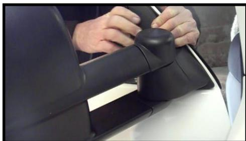
17. Screw in the top bolt first (initially not too tight) then the others. Then tighten all bolts.
